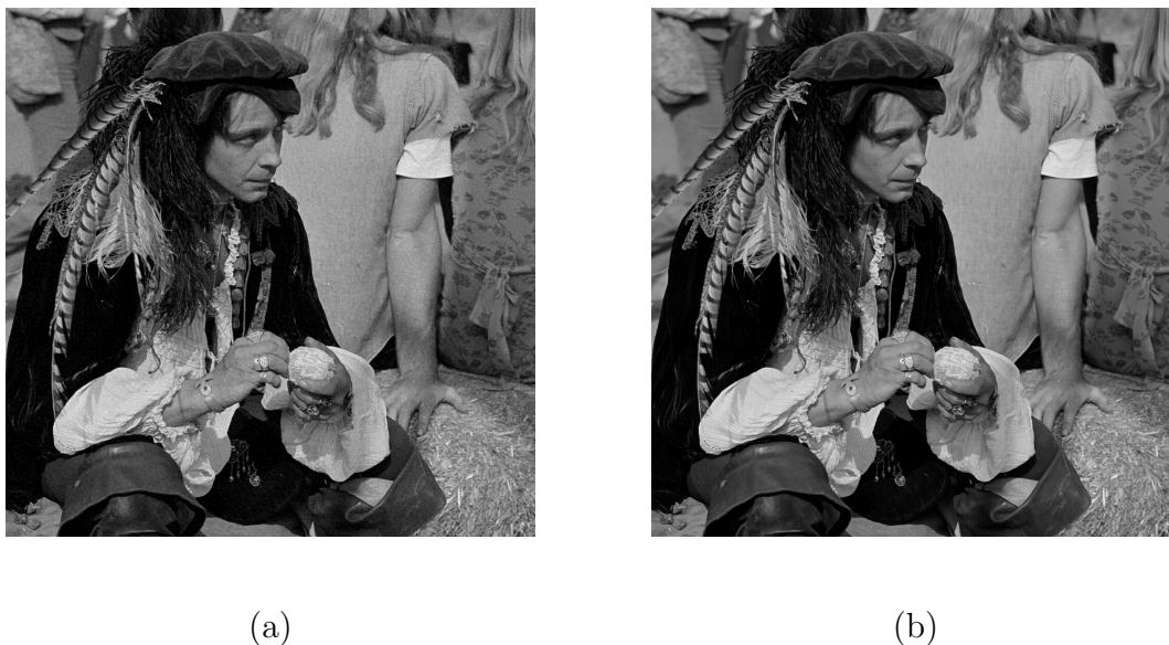
Figure 6.10: Illustration of a reversibility attack based on dither estimate according to Eq. (6.23). Image marked using \Lambda = E_8 , \alpha = 0.7 , p = 10 and PSNR = 38.2 dB (a), and estimate of the original image with PSNR = 55.9 dB (b).
