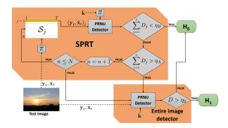
Fig. 1. Sequential test implementation.
